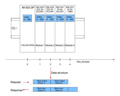
Each data block can be up to 244bytes. In the case of modular devices, the slot number is assigned to the modules. Compact devices are regarded as a unit of virtual modules. These can also be addressed whit slot number and index. Through the length specification in the read/write request, it is also possible to read/write parts of a data block.
