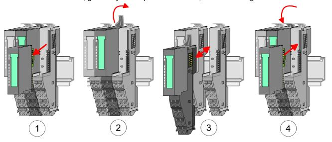
1 module group between 2 modules With mounting respectively de-mounting of a module group you also have to remove the electronic module of the just mounted <u>right</u> module! After mounting it may be plugged again.
