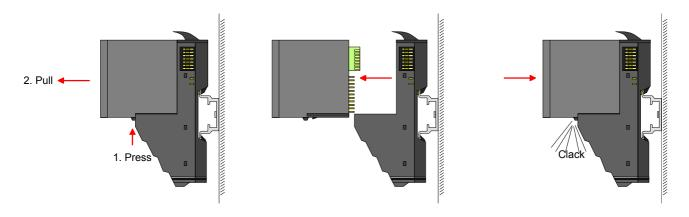
Mounting Proceeding The modules were directly be mounted to the mounting rail and so connected to the backplane bus and the power supply for the electronic and power section.
