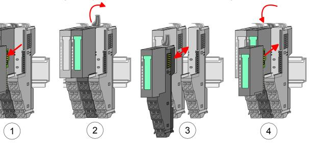
1 module group between 2 modules With mounting respectively de-mounting of a module group you also have to remove the electronic module of the just mounted <u>right</u> module! After mounting it may be plugged again.
