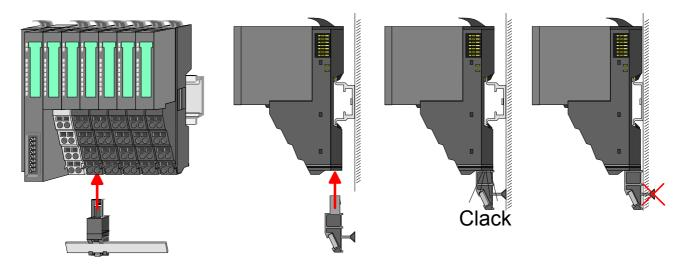
Mounting between 2 modules With the mounting of a FS200 module respectively of a group of FS200 modules between two modules for mounting reasons you have always to remove the electronic module of the just mounted <u>right</u> module. After that it may be plugged again.
