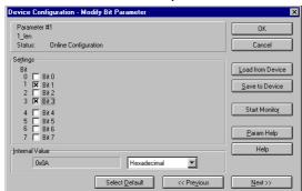
The analog module has 10Byte of parameter data. Enter this value as a bit-coded value.
